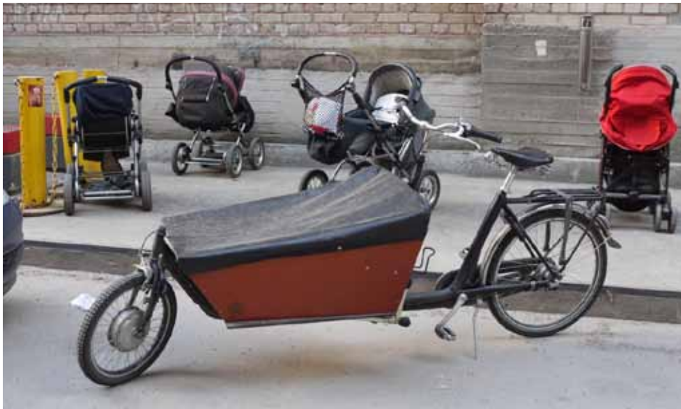
Figure 45. A bicycle equipped with a cargo box typical in Amsterdam. The version in the picture is a pedelec having the electric motor in the front wheel. Photo A. Alku 26.3.2011.
