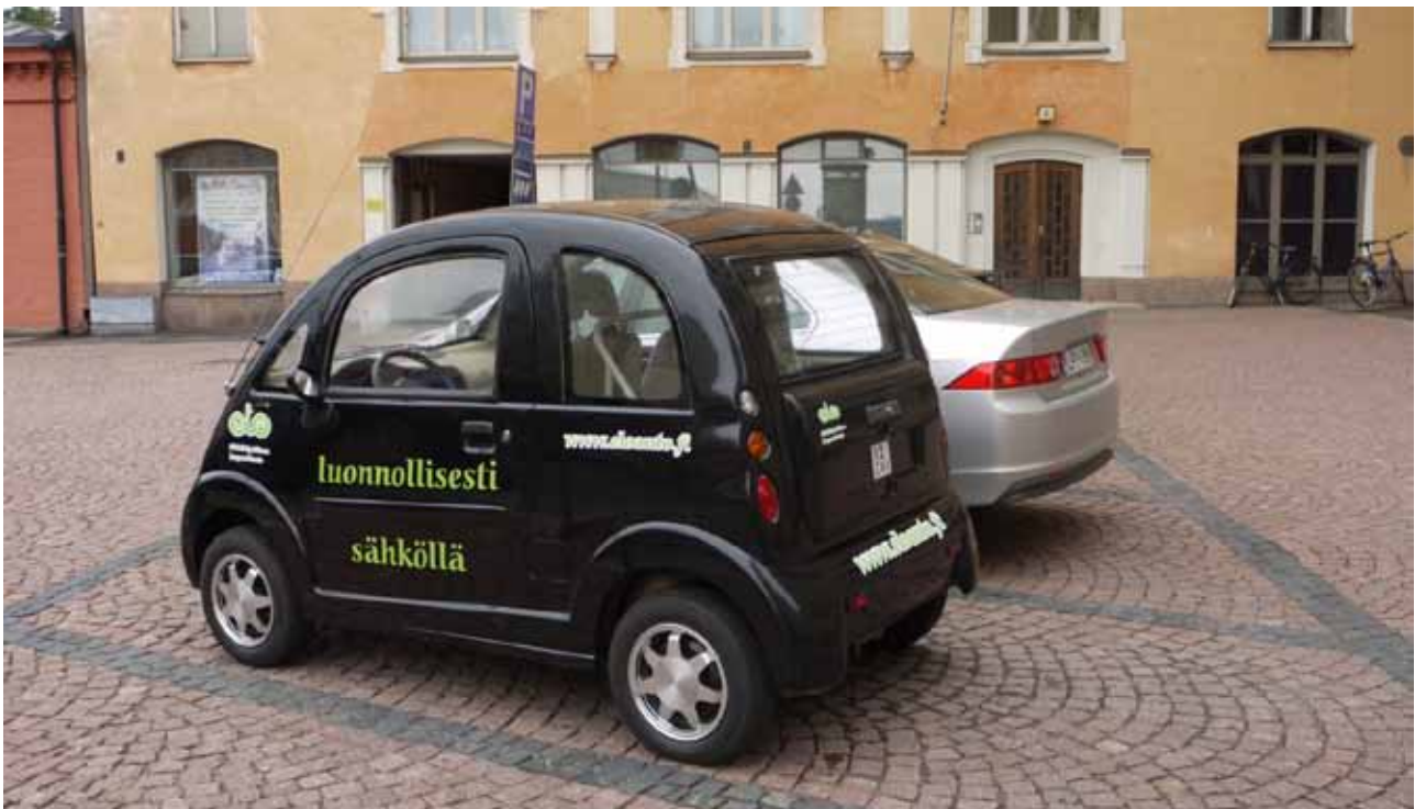
Figure 12. Electric quadricycle Elo, photo taken in summer 2010 in Helsinki. There is a moped insurance plate on the vehicle instead of normal registration plate.
