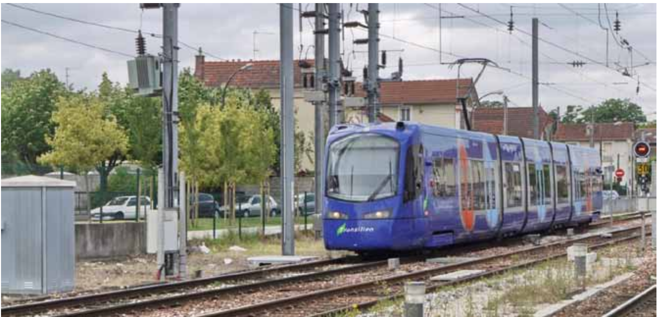
Figure 8. A tram-train on the Paris tram line T4 in June 2010. The Siemens-built Avanto S7 is composed of five units, with a total length of 36.5 meters.
