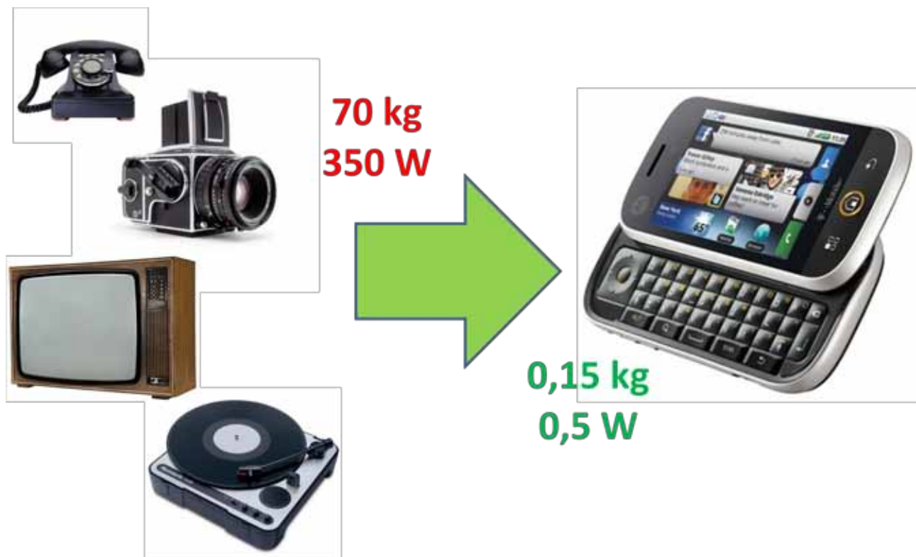
Figure 47. An example of a technological breakthrough, which has caused a total change in product concepts. Phones, cameras, televisions and record players were first turned into electronic and digital versions of the previous separate devices. Once their technology had become similar, they evolved into a new product concept, the smartphone. This evolution has reduced both the mass and the energy need of these devices.
